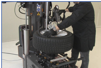
Montaggio tallone esterno Placement of external bead
