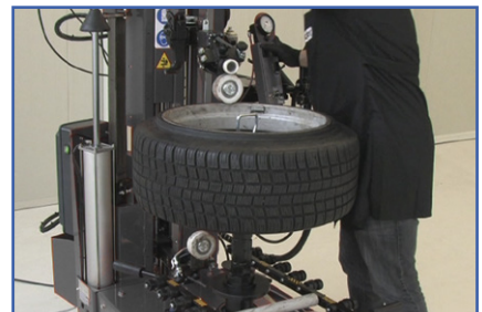
Fine montaggio PAX End of PAX system mounting
