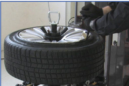
Distacco tallone esterno Demounting of external bead
