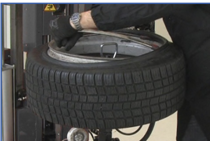
Sollevamento tallone lato interno Lifting of the second bead
