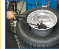
G1001.24AXIT G1005.ELIT Версии с бескамерной накачкой шин. Versions with tubeless tyre inflation system.
